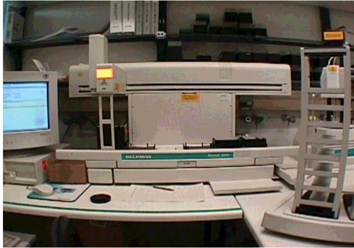
Figure 7: Beckman/Coulter Biomek 2000. A standard laboratory robot designed for liquid handling tasks.
